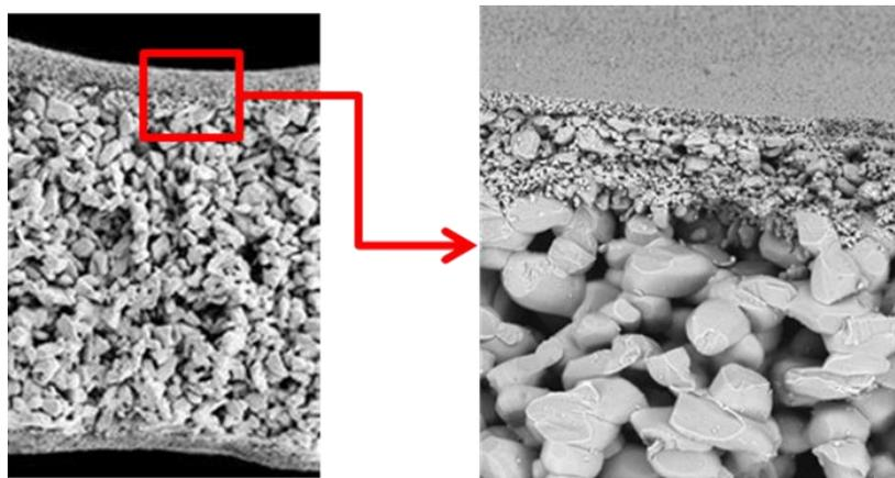
Figure 3: Cross-sectional view of Saint-Gobain SiC filter: coarse-grain carrier structure with fine-grain membrane layer.
