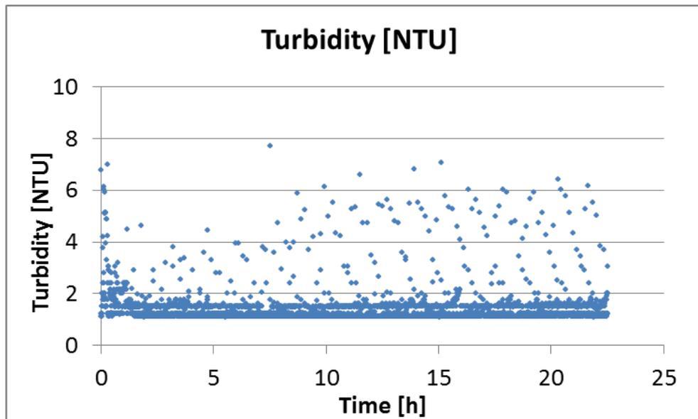
Figure 9: Typical turbidity evolution over the filtration cycle
